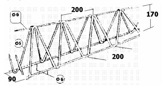
AB 90X170/200 \$\sigma 6 2 \$\sigma 5 L 2 \$\sigma 6\$ B500T 12 UNE 36739:1995 EX
